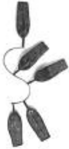
Curved wooden spline held in place by five weights.
